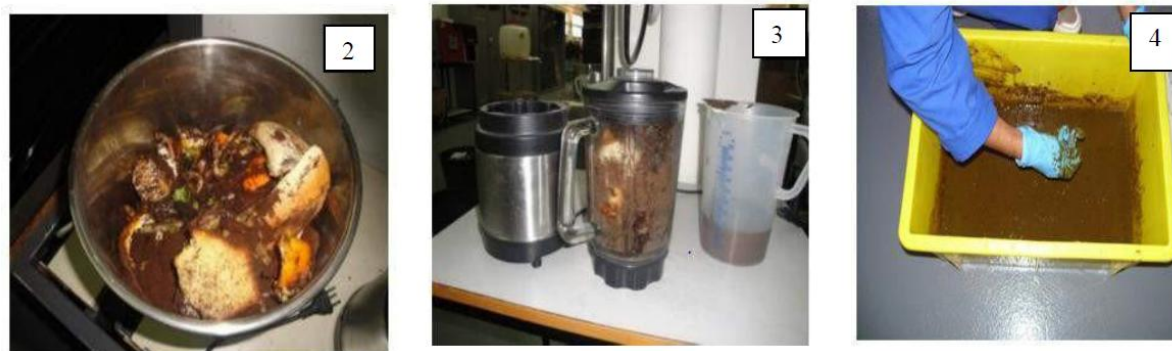
Figure 2, 3 & 4. Food waste taken from the canteen, made into a fine paste with biogas slurry from WWTP and cow dung slurry
